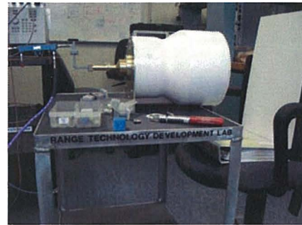
NDE/I CUP Test Set Laboratory Prototype with painted steel test exemplar
