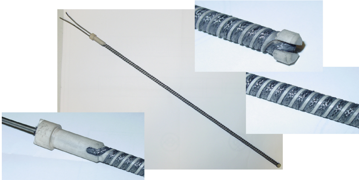
Figure 20. Carbonized C fiber braid wrapped in a double helix fashion around \text{Al}_2\text{O}_3 mandrel.
