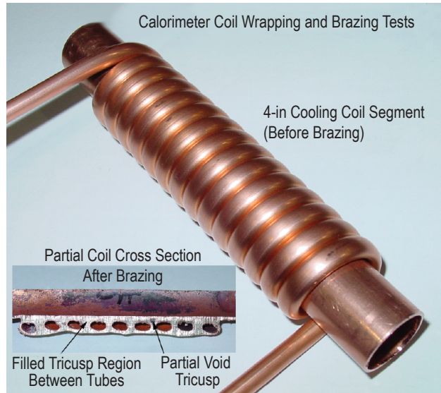
Figure 47. Calorimeter coil fabrication tests.
