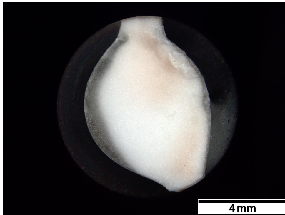
Figure 6. Penetration of surface discoloration into the insulator cross sectional thickness. (10x)
