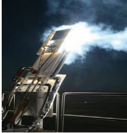
Figure 228. Solar tower test of ablator panel.
