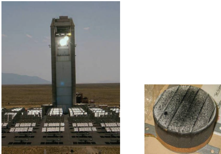
Figure 227. Solar tower test of ablator coupons
