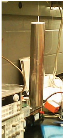
Figure 153. Test cylinder with the heating element running down the center and sheathed with an alumina tube. It was found the alumina tube would melt and destroy the test apparatus.
