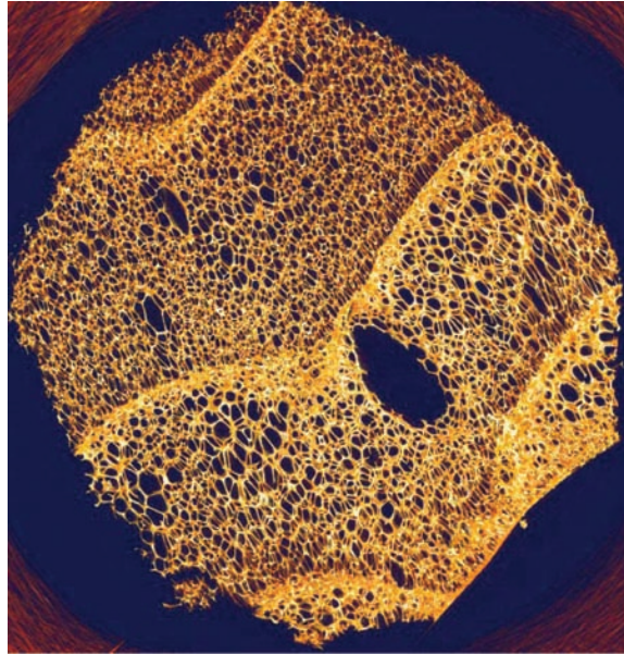
Figure 49. Phase contrast tomographic image showing intact foam structure and defects inside a foam insulation region at and near the interface between the foam and the Al substrate.
