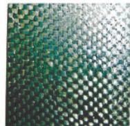
Figure 198. Pretest photograph of carbon/PBZ composite specimen.
