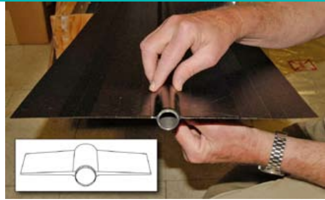
Models showed that heat pipes with tapered, wafer-thin, coated fins would provide greater heat rejection and would result in a decrease in radiator weight and size.
