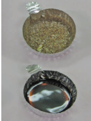
Figure 132. Two polyimide films: (1) CP2, a conventional material (top) developed at LaRC and (2) ILPI-1, an IL-based material (bottom) developed at MSFC. Note that the IL polyimide contains fewer bubbles/voids that can reduce mechanical strength. This probably occurs because the IL polyimides are more mobile at high temperatures, thus the water vapor is able to escape much easier.
