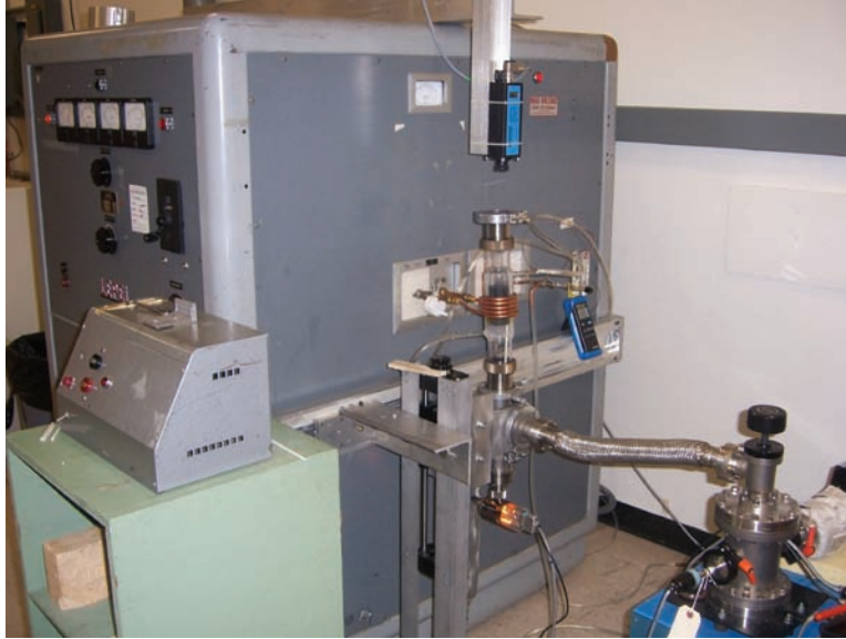
Figure 81. High-temperature crystal growth and materials processing facility.
