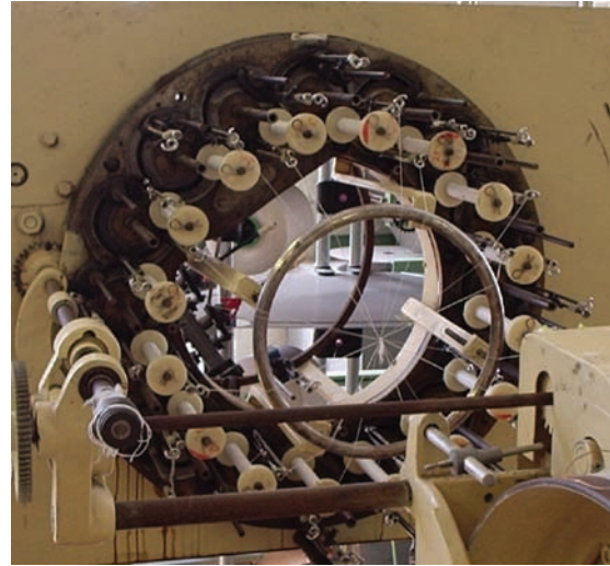
Figure 87. Thirty-two carrier braider used for combining fiber optic with ZYLON and Al.
