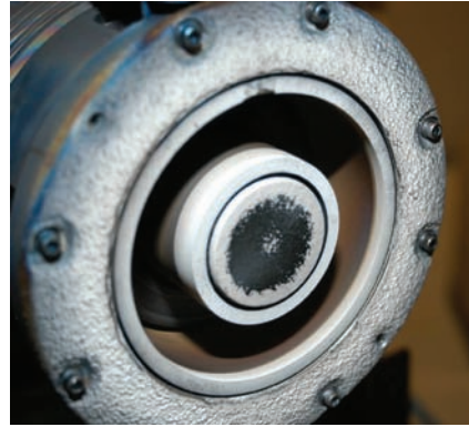
Figure 75. Characteristic erosion of Hall-effect thruster (NASA GRC).
