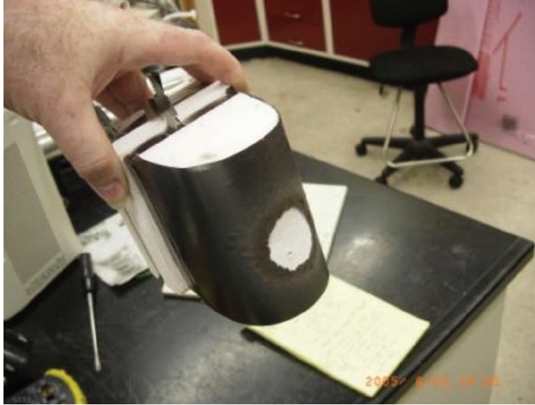
Figure 174. First torch test article of Grafoil (C) shaped over insulating brick. Lifetime of target was very limited and offered no measure of bias effects.
