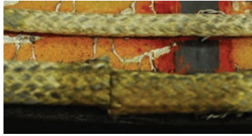
Figure 18. Typical area of rope seal. Figure 19. Outer rope-seal joint. Figure 20. Inner rope-seal joint.
