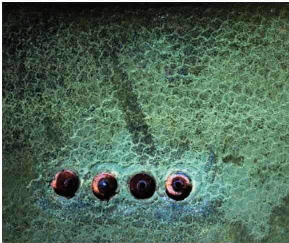
Figure 16. Plugs (located at \approx 240^\circ ) surrounding blue-green areas indicate outgassing from RTV materials.
