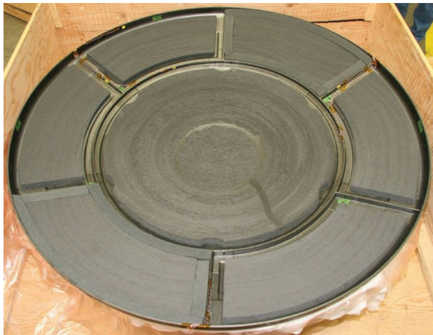
Figure 167. Same view as figure 166, but Calcarb Ltd. carbon fiber insulation is installed.
