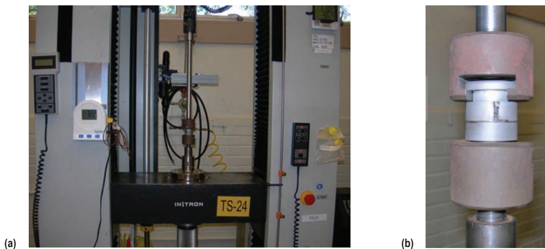
Figure 131. Preparation of Al button samples and adhesive tensile testing using an Instron machine.
