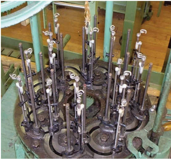
Figure 86. Sixteen carrier Wardwell braider used for 16 package configurations.
