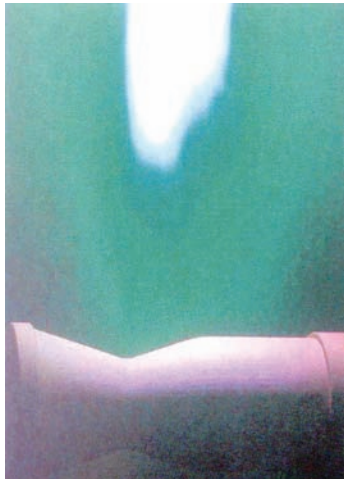
Figure 55. To make a thrust chamber liner with VPS, materials are deposited on a mandrel to form a near-net shaped part. This process is being developed to provide durable, robust, high-temperature protective coatings for propulsion engine components.
