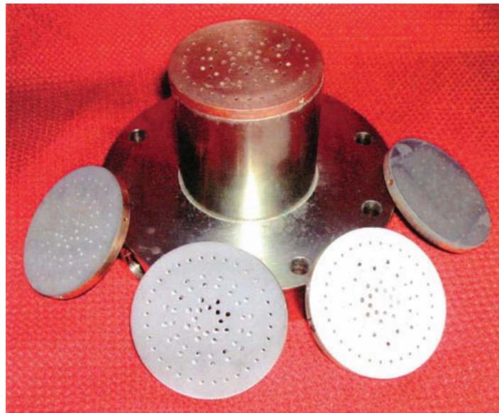
Figure 63. Injector fabrication—Four coating options applied to injector designs.
