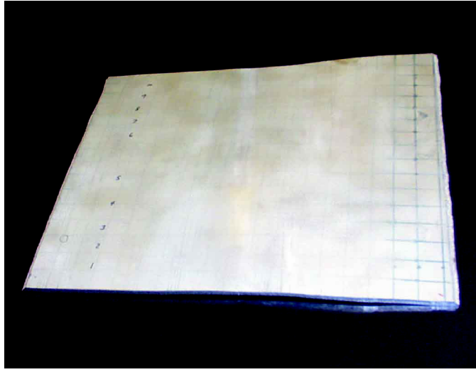
Figure 12. S/N 007 debuckled test section.
