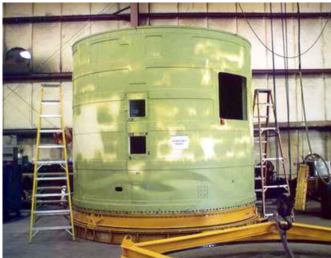
Figure 1. S/N 20022 buckled forward skirt.
