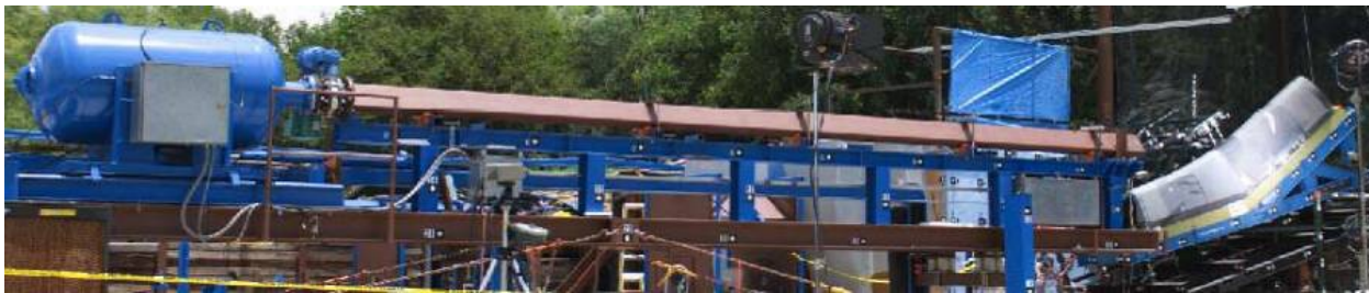
Figure 8. Ballistic Impact Test with a Full-scale Wing Leading Edge Test Article.
