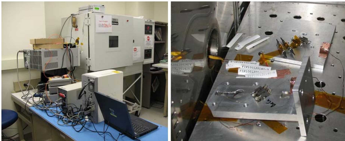
Figure 7: Thermal Cycling Testing Set-up with Insitu Optical Power Transmission Monitoring of Mini AVIM and DMI Interconnection.
