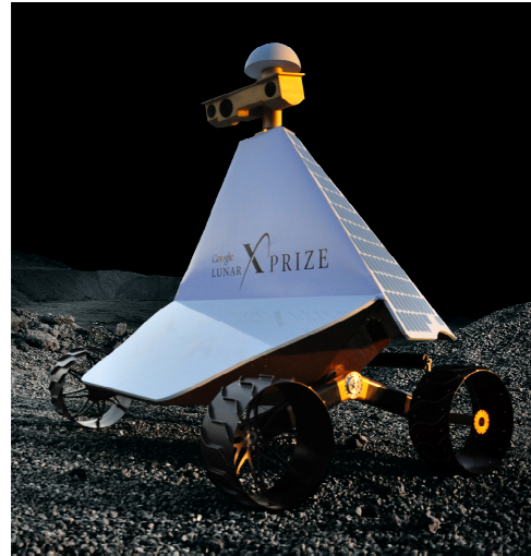
Figure 2.—Asymmetric rover for operation during the heat of the lunar equatorial day.
