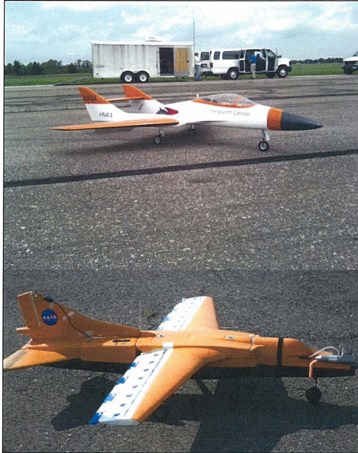
FIGURE 28: JET POWERED (JFLIC) AND INTERNAL COMBUSTION POWERED (FLIC), FLYING CONTROL TEST BEDS WITH GROUND CONTROL STATION IN BACKGROUND
