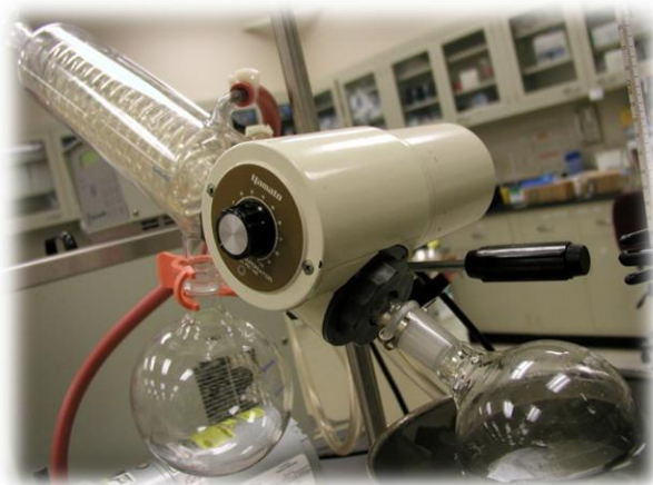
Figure 5: Image of the rotary evaporator used in the synthesis of IL systems
