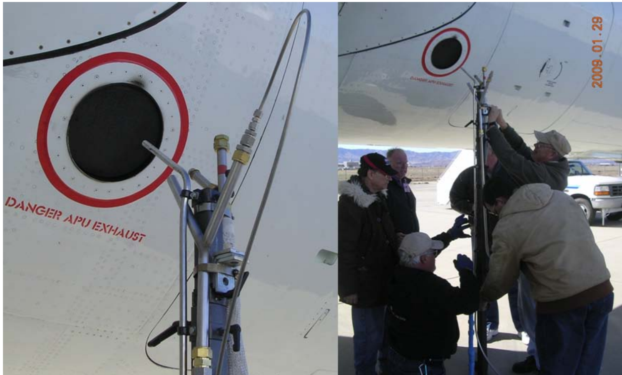
Figure 14. The photo on the right shows the inlet probes used for sampling exhaust from the DC-8 APU. On the left, members of the AAFEX science team erect the inlet stand and adjust its position to align the probes with the exhaust flow.
