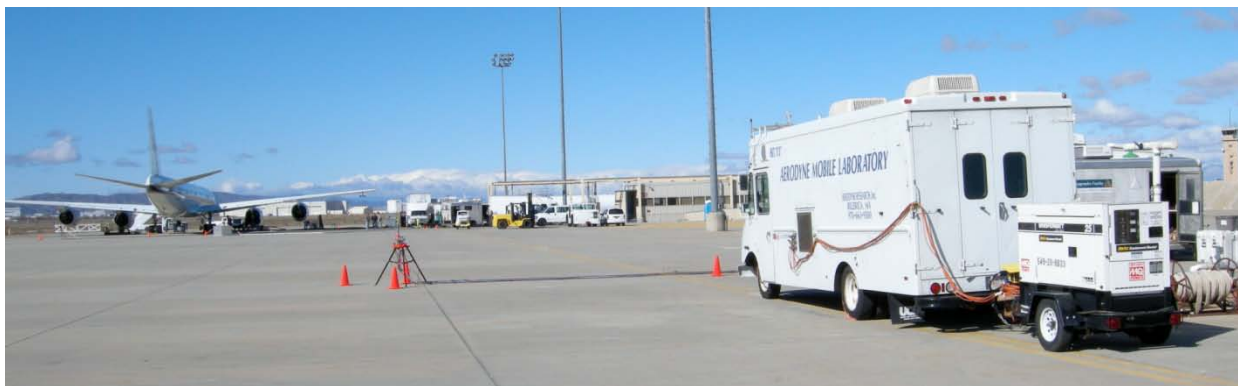
Figure 13. ARI mobile laboratory with diesel generator hitched to the back.
