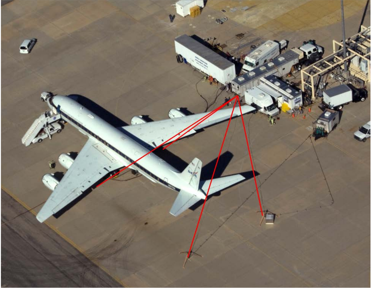
Figure 1. DC-8 with red lines superimposed showing the four sampling lines used to transport exhaust from the 1- and 30-m inlets to the sample distribution manifold located in the MST trailer.
