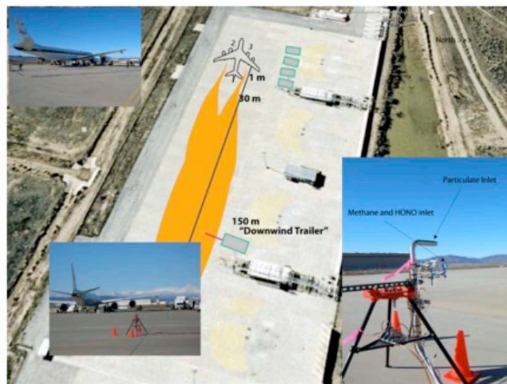
Figure 1: AAFEX sampling layout and the 145 m "advected-plume" trailer positioning relative to the aircraft
