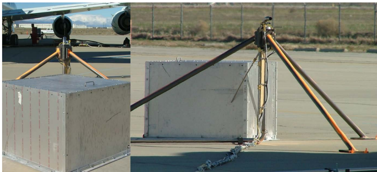
Figure 11. R30 with the "Death-box" instrument enclosure bolted to the tarmac immediately downstream.
