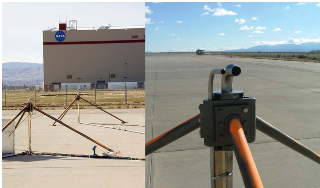
Figure 9. At left, the identical inlet probes and tripod stands used to sample exhaust emissions at 30-m behind the DC-8's #2 and #3 engines. The image at right shows the 1.9- and 5-cm inlet tubes used to deliver sample to the community aerosol sample manifold and EPA trailer, respectively.
