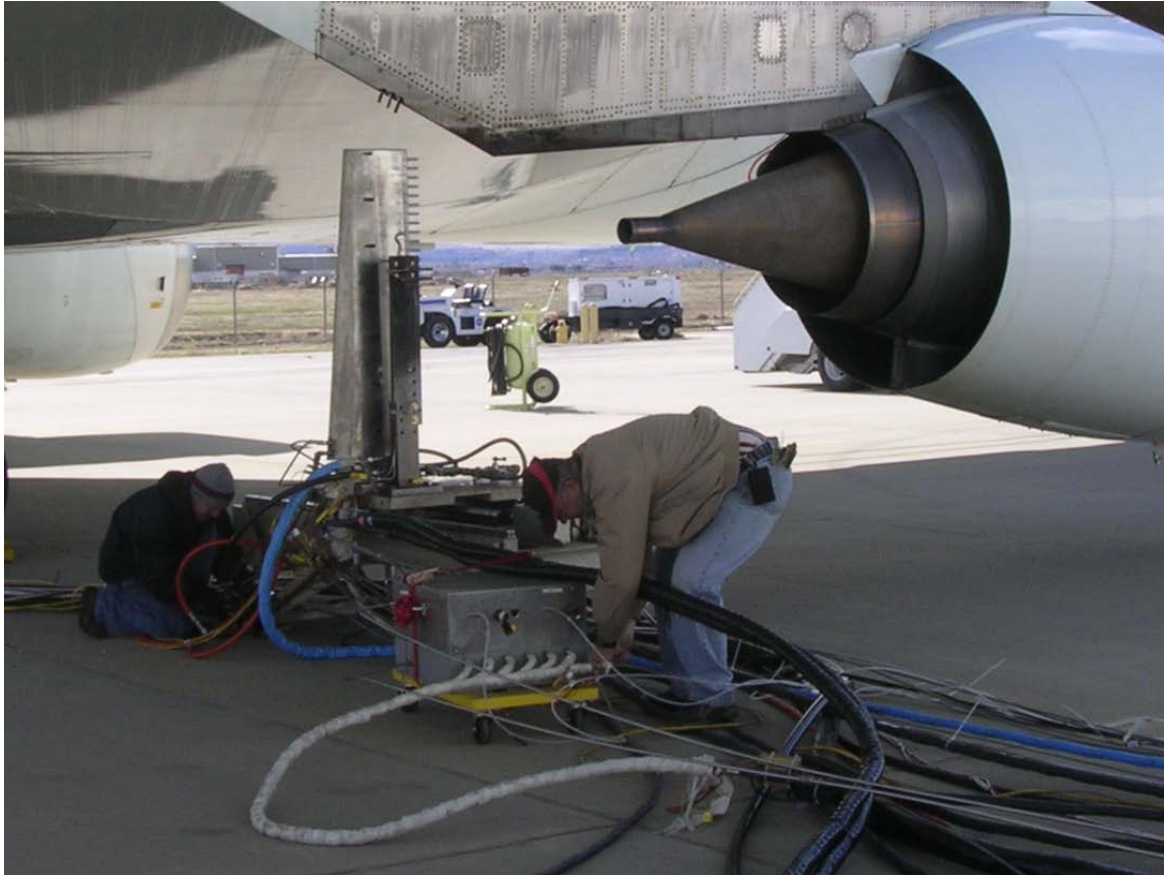
Figure 6. The traversing rake (R1) used to sample emissions behind the right inboard (#3) engine.
