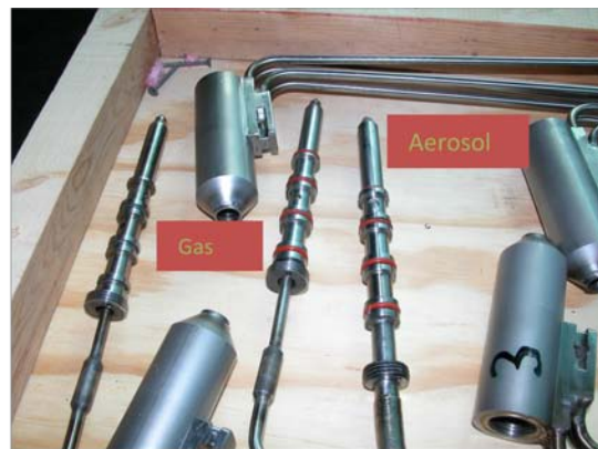
Figure 7. At left, cross-sectional diagram of AEDC dilution probe showing the sample, water and diluents flow paths around the inlet tip. APEX-1 style gas and aerosol inlet probes used in L1 shown at right.
