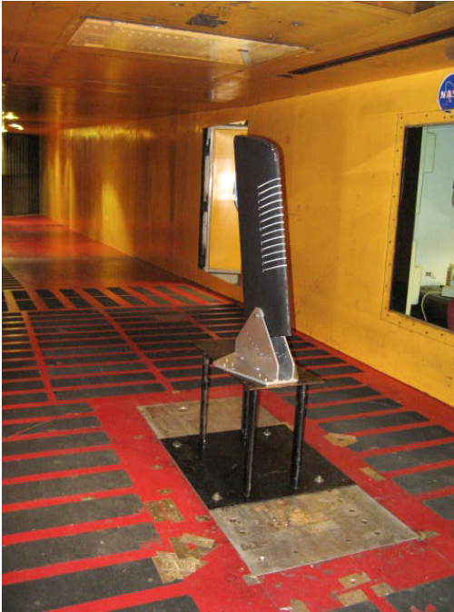
Figure 1.—Wooden NACA 0012 swept wing tip in the IRT test section.
