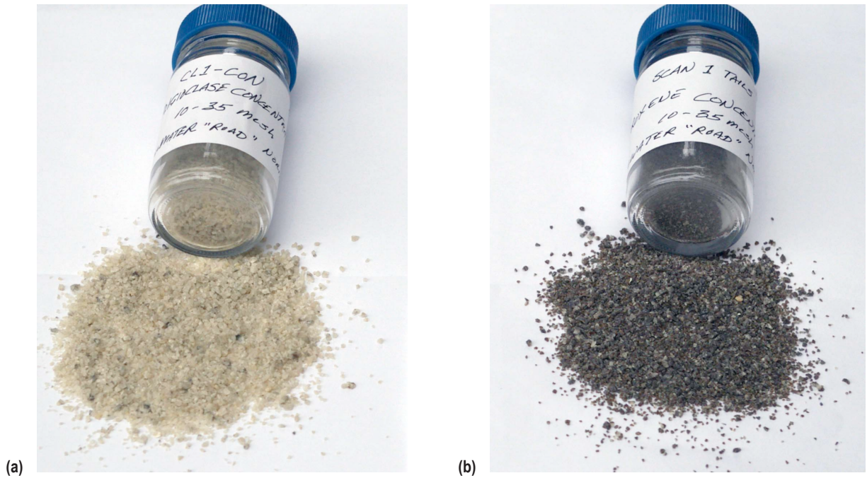
Figure 32. The concentrate 32(a) and tails 32(b) from the 10–35-mesh fraction as processed according to figure 30.
