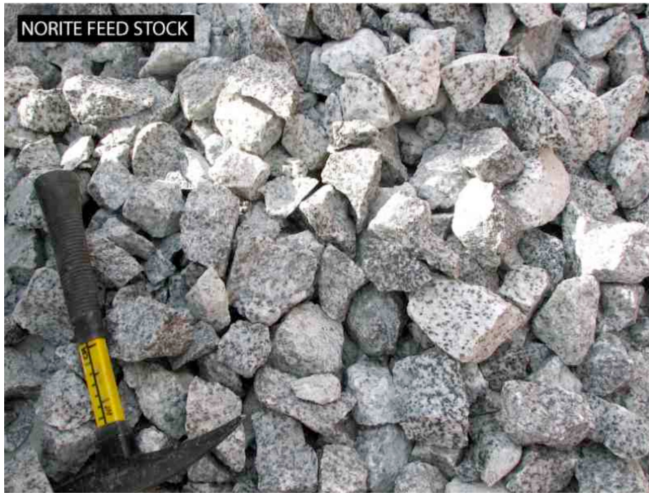
Figure 27. Norite after first stage crushing. Note the wide range in color variation. This is a result of both variations in the relative abundance of pyroxenes and the amount of hydrothermal alteration. (Courtesy of USGS).
