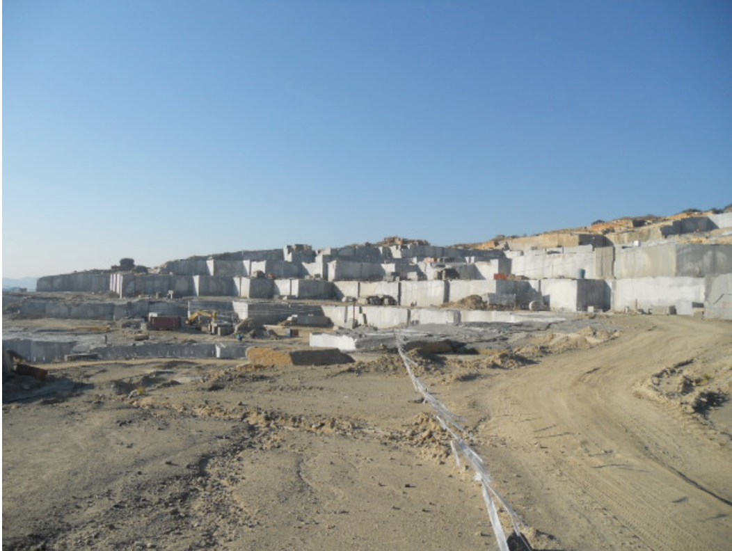
Figure 40. A quarry that produces the dimension stone Impala Black. This is but one of many quarries operated by M+Q and producing this specific stone. Image by Jonathan Houghton.
