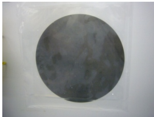
Figure 9.—MEA with platinum-black catalyst on hydrogen side and iridium oxide catalyst on oxygen side.
