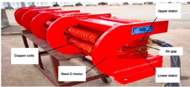
Fig. 1. 300 Hz Double-sided linear induction motor (DSLIM) with two stators mounted in a C-frame.
