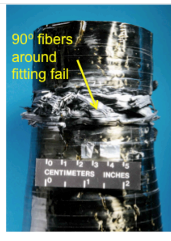
Fig. 30. Failure of a corrugated fitting strut.
