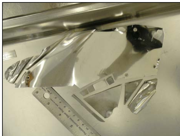
Fig. 1. Overview image of the remaining polished aluminum kidney after the most recent subdivision.
