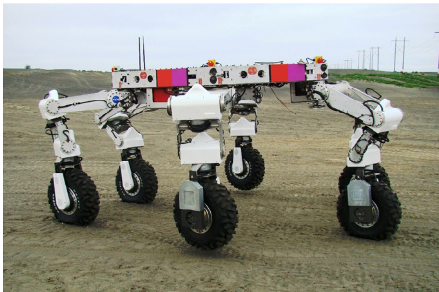
Figure 13: ATHLETE Robot. This prototype is an appropriate scale for conversion to a lunar hopper with scavenged RCS thrusters. (Photo R. Oeftering)
