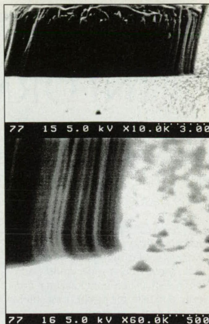
Figure 2. The Scanning Electron Micrographs show two views of the sidewall of a mesa etched around a masked area by an atomic beam incident a few degrees off perpendicular from the surface. The bottom panel is an enlarged view of the lower right region of the same sidewall that is seen in the top panel. The fluted appearance of the wall is attributed to the rough edge of the mask.
