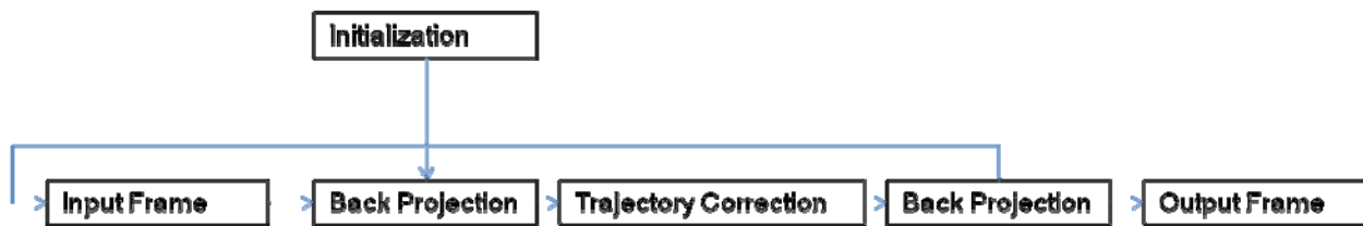
Figure 2: Block diagram of the computer code implemented super-resolution method
