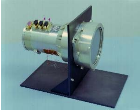
Figure 1. NaI(Tl) detector with viewing angle, \phi , between the yellow source vector and the
