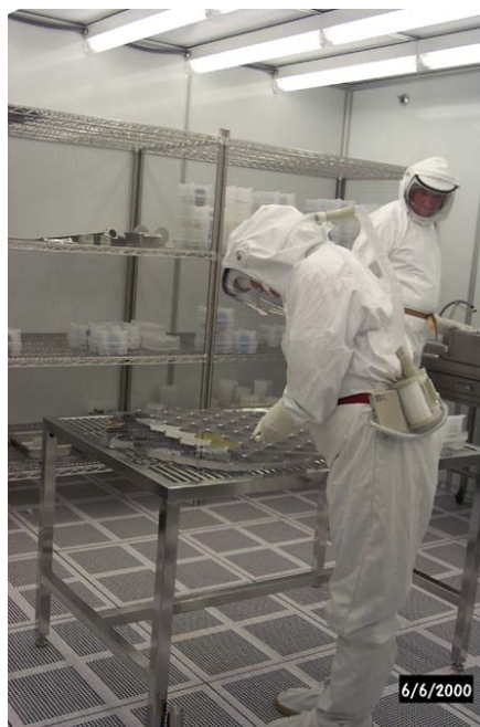
Fig. 1. Assembly of Genesis collectors in ISO Class 4 cleanroom at Johnson Space Center. Workers are enclosed in Teflon suits with HEPA-filtered exhaust.
