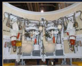
Same Aft Skirt and Thrust Vector Control as Shuttle
