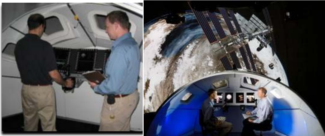
Figure 2. The ROC facility, where the left photo shows the actual setup (illuminated by the camera flash) and the right photo show an example of out-the-window scene generation.
