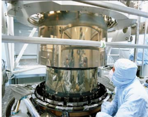
FIGURE 2. The cartoon on the left illustrates the principal of grazing incidence which allows X-rays to reflect as long as the angle of incidence is below the (energy-dependent) critical angle. The picture on the right was taken at the Eastman Kodak tower where the optics were assembled and aligned. The iridium coating is on the inside of the reflecting cylinders of revolution.
