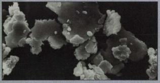
Novamet HCA-1 Flake, screen mesh 98% minus 400, apparent density 0.90 g/cc, thickness 1.0-1.1 microns, surface resistivity 0.25  $\Omega/\Box$ .
