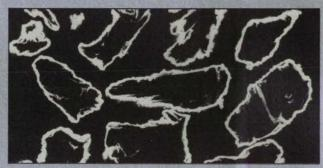
Novamet Nickel Coated Graphite, 60% fully encapsulated Ni, apparent density 1.6 g/cc, particle size (FSSS) 100 microns, screen mesh 63% - 150/ + 250, surface resistivity 0.3  $\Omega/\Box$ .
