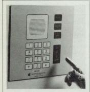
Designed to reduce clean room contamination caused by traditional telephones, the **Model 295 Clean Phone** from GAI-Tronics Corp., Reading, PA, features a smooth, crevice-free front panel and an integral speaker/microphone. The microprocessor-based phone offers remote programming for two autodial numbers, call timeout, and auto answering and is available in flush- or wall-mount styles.
