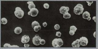
Novamet Silver Coated Nickel Spheres, 15% Ag, 2.5 g/cc apparent density, particle size 10 microns, screen mesh 99%-250, surface resistivity 0.03  $\Omega/\Box$ .
