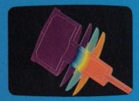
Transient heat transfer by direct integration-2D and 3D elements; animated contours Part 106 adds to Part 101 or 102 \$300
