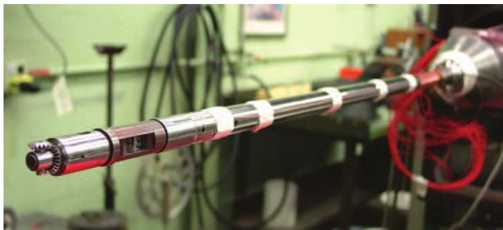
Figure 4. Internal strain-gauge balance used during the wind tunnel tests at PSWT.
