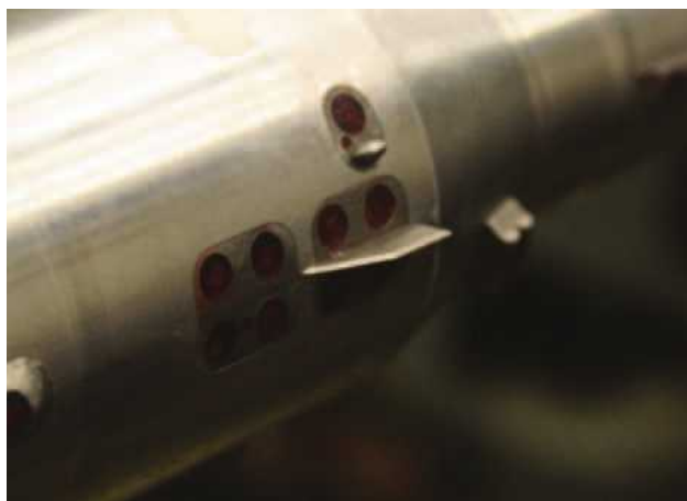
Figure 12. Picture of one of the aerodynamic strakes on the wind tunnel model utilized to mitigate rolling moment.
