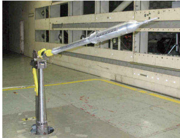
Figure 6. Model installation in 14x22 SWT for transition test.
