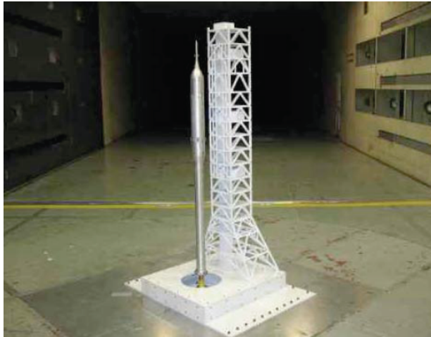
Figure 5. Test model with tower in 14x22 SWT.
