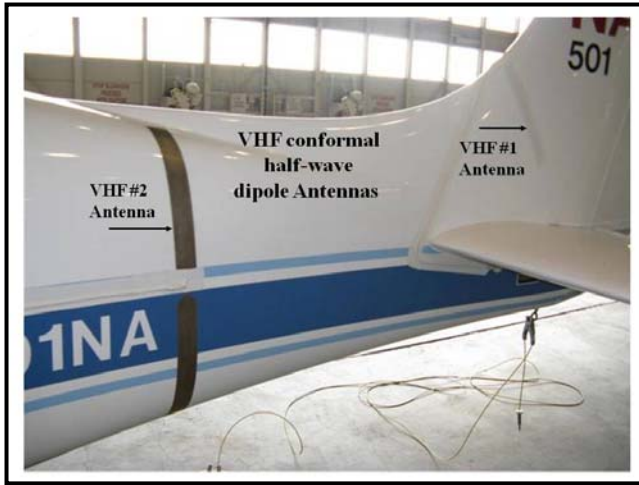
Figure 5. VHF Half-Wave Dipole Antennas
