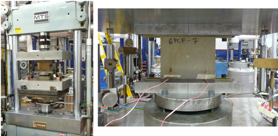
Figure 7. Compression after impact test apparatus.
