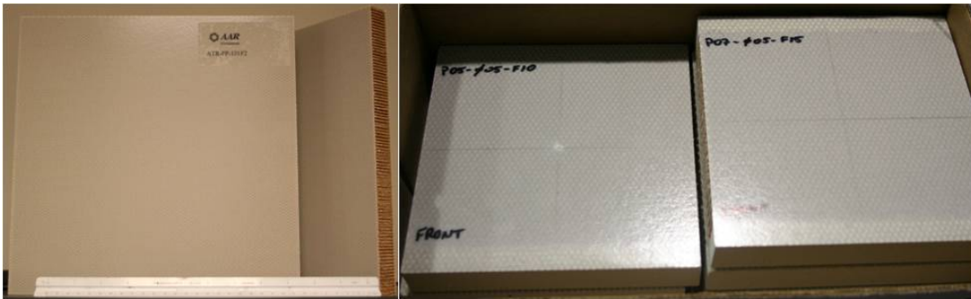
Figure 1. PXX sandwich panel material (left) and PXX material coupons (right).
