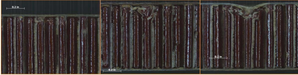
Figure 6. Examples of interior damage images at 1.0 (left), 3.0 (center), and 5.0 (right) ft-lbs. for 6PCF type sandwich panel construction.
