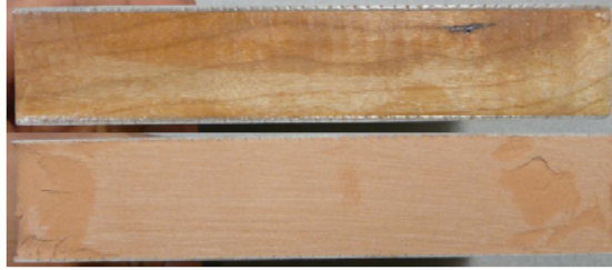
Figure 2. Comparison of wood filled (top) and potting material filled (bottom) coupon ends.
