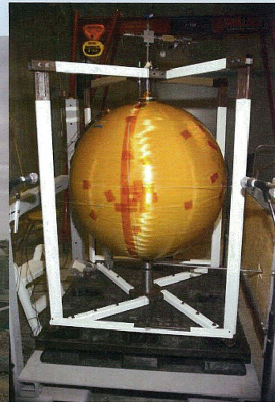
OMS/RCS test article in test frame. Allows freedom of movement to monitor vessel dimensional changes during test.
