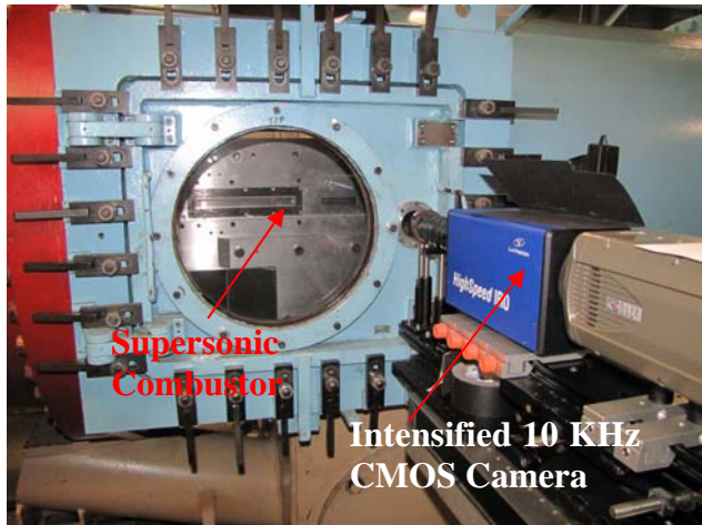
Figure 5: Photograph of generic Scramjet engine model and Intensified CMOS camera system.
