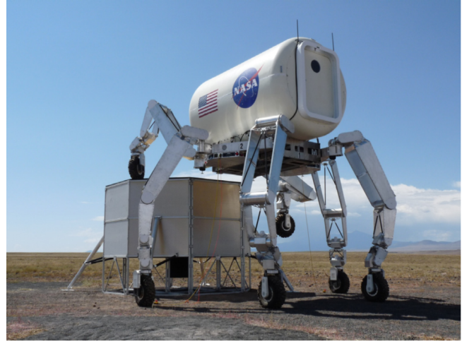
Figure 2. The next generation of ATHLETE, T12, is two Tri-ATHLETEs docked to a pallet. Here, T12 carries a simulated astronaut habitat while walking off a simulated lander. T12 has seven degrees of freedom in each leg and many sources of compliance all over the robot. Picture by JPL.
