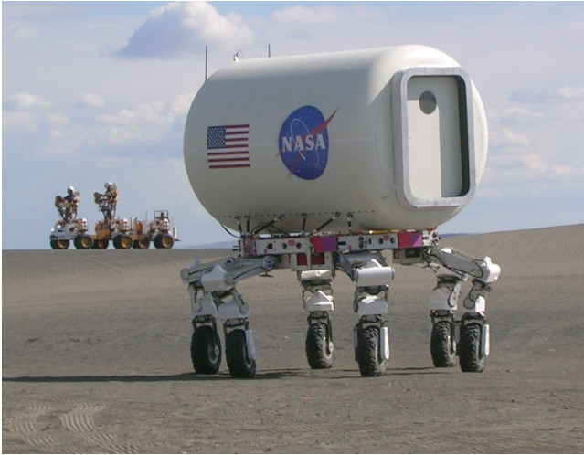
Figure 1. The original ATHLETE robot, SDM-B, carrying a simulated astronaut habitat. ATHLETE has six degrees of freedom in each limb and most of its compliance comes from the tires. Picture by JPL.
