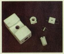
Mykroy/Mycalex Grade 561 high-temperature glass-bonded ceramic material from Spaulding Composites, Rochester, NH, is a mica ceramic that withstands operating temperatures to 1400°F. The material offers dimensional stability, the ability to hold metal inserts in
