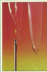
Stevens Urethane, Holyoke, MA, has introduced two grades of flameresistant **thermoplastic polyurethane.** The ST-1796 and ST-1776 meet UL-94-VTM-O standards for flame-resistance and are designed for applications requiring flameresistant thin films. ST-1796 features a standard VTM-O package using an antimony oxide synergist with halogen-based flame retardant; the ST-1776 features an alternate non-halogen FR system.
