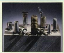
ND Industries, Troy, MI, offers Plastisol PVC liquid vinyl dispersion material that can be fused to a fastener by externally applied heat. When applied heat. When applied on the underside of a variety of rivets, it seals against air, water, and dirt, and absorbs noise and vibration. The materi-
