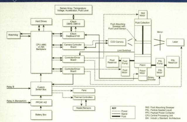
Figure 1. Inside the Get-Away Special Vortex Experiment Instrumentation.
