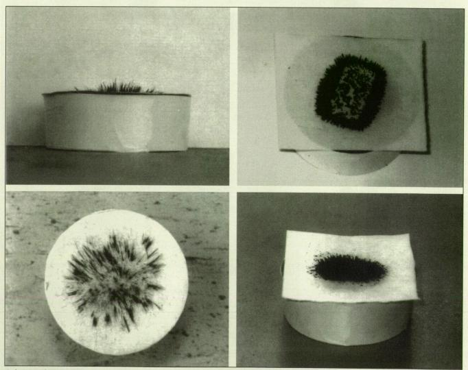
Carbon-Based Material That Contains  $Fe_3O_4$  becomes arranged in the familiar pattern of magnetic-field lines when placed on the face of a permanent magnet. On the left are side and top views of a fibrous sample; on the right are two angle views of a powdered sample.
