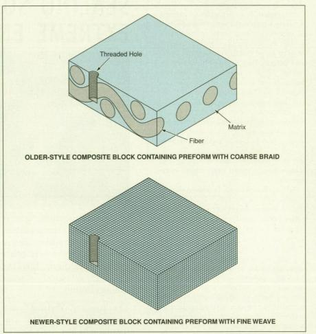
The **Fine Weave** of the newer composite is more conducive to fine machining and to retention of strength in fine details like screw threads.
