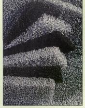
Goodfellow Corporation, Berwyn, PA, has introduced an **aluminum alloy foam** made of alloy 6101. The true metal foam is similar to natural sponge in appearance, yet retains its alloy characteristics. It is corrosion-resistant, intrinsically strong, and is thermally and electrically conductive. The foam offers low density of 0.08 to 0.32 g/cm<sup>-3</sup>, of which 3 to 12 percent is solid aluminum.
