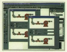
format logic control software that manages control tasks such as loading, starting, and basic diagnostics.
