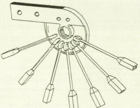
DETAIL OF END FITTINGS IN SLOTS IN DEPLOYED POSITION
