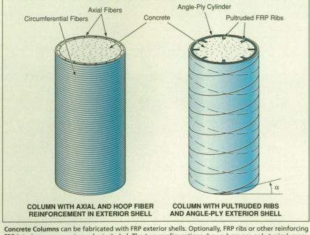
**Concrete Columns** can be fabricated with FRP exterior shells. Optionally, FRP ribs or other reinforcing FRP interior components can be included. The two configurations shown here are only typical; many other configurations are also possible.
