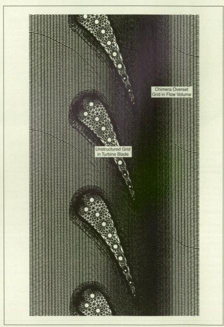
A **Chimera/Unstructured Hybrid Grid** enables the computational treatment of a turbine cascade as one integral system, for which the coupled equations of aerodynamic, thermal, and structural effects can be solved together.
