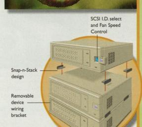
Kingston's new cost effective Data Stacker<sup>™</sup> can adapt to your changing storage needs just as smoothly and easily as the chameleon adapts to its changing environment. With Data Stacker's Snap-n-Stack design, it's simple to pop-on or off units effortlessly as your storage requirements change.
