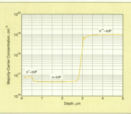
The Majority-Carrier Concentration of a specimen of n<sup>-</sup>-doped InP deposited on n-doped InP deposited on n<sup>+-</sup>-doped InP substrate was determined by electrochemical profiling in the UNIEL solution.
