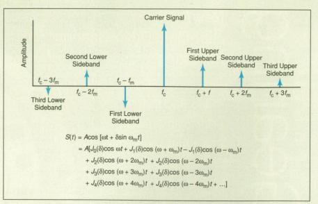
Figure 1. The **Spectral Symmetry** of a phase-modulated signal precludes extraction of amplitude modulation via beat notes and simple detection. Here *S* is the instantaneous signal amplitude, *t* is time,  $\omega = 2\pi f_c$  where  $f_c$  is the carrier frequency,  $\omega_m = 2\pi f_m$ ,  $\delta$  is the maximum phase deviation, and  $J_i$  (*i* an integer) denotes a Bessel function.
