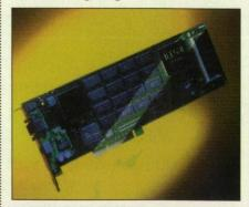
coordinate generation, and fog calculation. It is configured with a 16-MB VRAM frame buffer and 24 MB DRAM expandable to 40 MB - local buffer memory for Z-buffering and texture mapping. It supports high-resolution, true-color display of up to 1920 x 1080 or 1600 x 1280 on 24" monitors.
