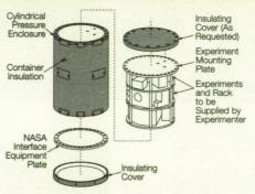
Figure 2. Get-Away Special Small Self-Contained Payload Container Concept.
