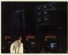
Denver International uses CTAS to help controllers manage air traffic more efficiently. CTAS data is displayed via overhead projectors, allowing controllers to view the information while working at their radar stations.
