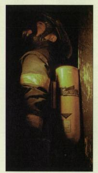
The NASA-developed breathing system was designed with a reduced profile to improve mobility when firefighters are required to squeeze through narrow areas.
