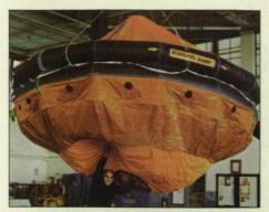
The hemispheric underside of the Givens Buoy Raft is designed to prevent capsizing in rough water. The design is similar to that of a NASA raft developed for astronaut recovery after ocean landings.
