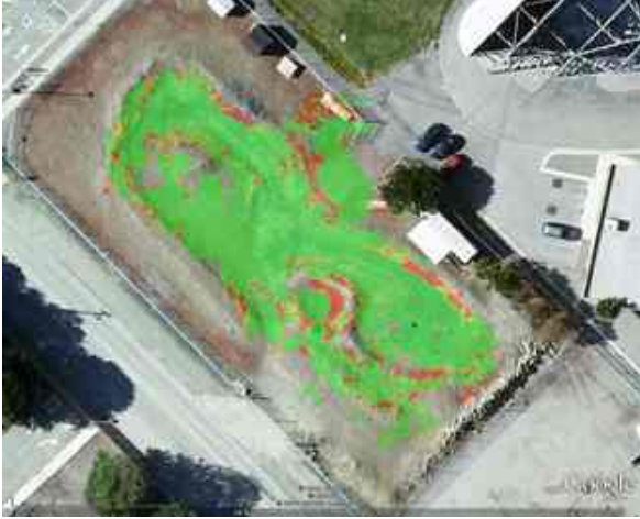
Figure 6. : Time Windowed Morphin traversability map. Green areas have slopes < 13^\circ , red areas have slopes > 23^\circ .
