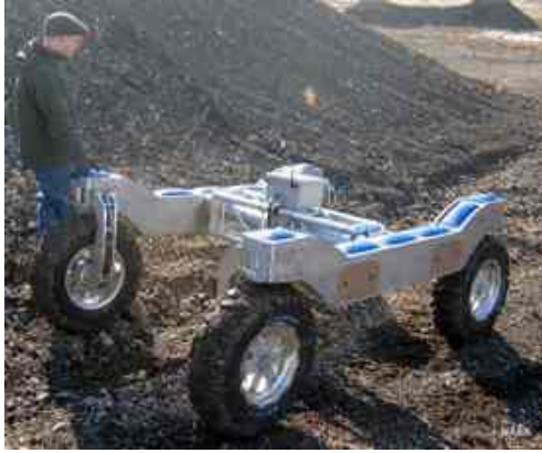
Figure 3. : The Lunar All Terrain Utility Vehicle (LATUV), developed by ProtoInnovations LLC under a NASA SBIR as a research platform for lunar navigation and capable of speeds up to 2m/s.
