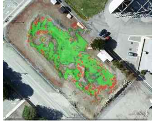
Figure 7. : Probabilistic Terrain Analysis (PTA). The red areas have confirmed obstacles at least 10cm high. Areas with sufficient measurements but no obstacles are labelled traversable (green).
