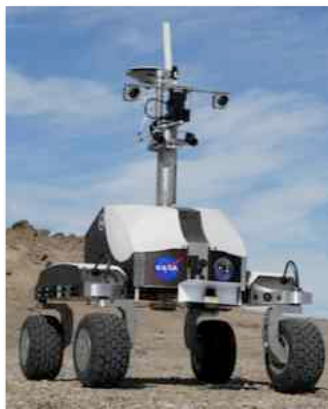
Figure 2. : NASA's K10 rover, an autonomous or tele-operated robot designed for robotic site survey [3] at speeds up to 0.6 m/s
