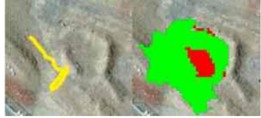
Figure 9. : Occlusion map of a crater generated as the K10 rover drives towards it on the indicated path (occluded areas are red).
