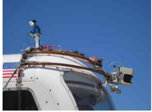
Figure 5. : Terrain mapping, hazard detection and pose estimation sensors on the LER
