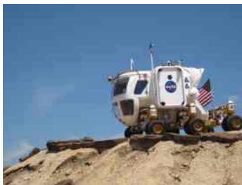
Figure 1. : NASA's Lunar Electric Vehicle (LER), designed to sustain a 2 person crew and drive at 3m/s on rough terrain
