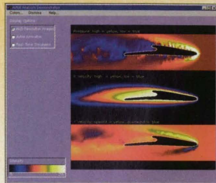
The flow of a wind tunnel is shown in this airfoil analysis performed with PV-WAVE from Visual Numerics.
