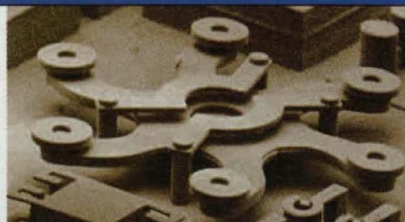
EFAB enables fabrication of micro-parts like this array of spray nozzles for a fuel injector. The CAD image used to design the parts is shown on the left. The actual nozzle array, pictured on the right, measures 2 mm across.
