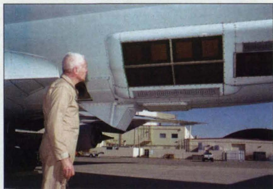
Pilot Edwin Lewis inspects the antenna for the Airsar instrument, mounted behind the wing on NASA's DC-8 airborne lab.
