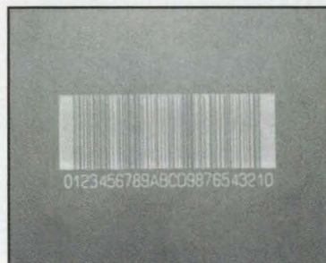
Using a Synrad 25 watt marking system, these codes were marked at 250" per second!
