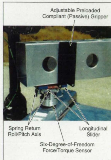
Figure 1. The Gimbal Mechanism enables the gripper to move freely in one translational and three rotational degrees of freedom, and measures forces and torques.
