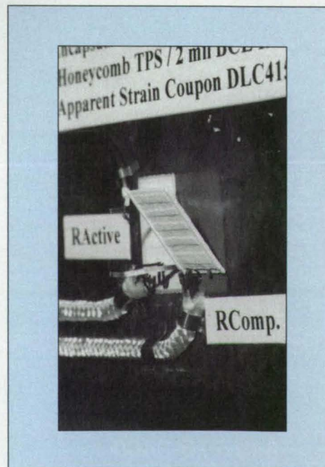
Figure 1. The Active Strain Gauge and the Temperature-Compensation Element are labeled "RActive" and "RComp," respectively. The straps that hold down the compensation element have been removed, and the gauge has been lifted for this photograph. Contact with the substrate must be maintained to ensure thermal conduction in the presence of transient heating.
