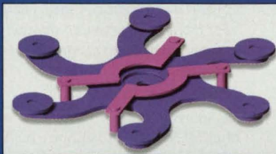
EFAB enables fabrication of micro-parts like this array of spray nozzles for a fuel injector. The CAD image used to design the parts is shown on the left. The actual nozzle array, pictured on the right, measures 2 mm across.
