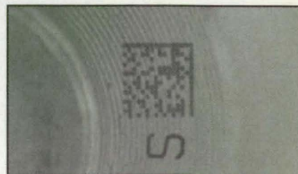
The Data Matrix™ Code (~0.2" sq.) on this torque converter was marked using WinMark Pro's Spot tool. The code was marked with 95 watts of power at a speed of 1" per second (7.4 second cycle time).
