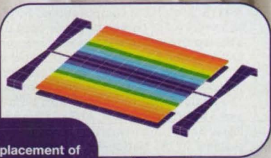
Displacement of MEMS switch
