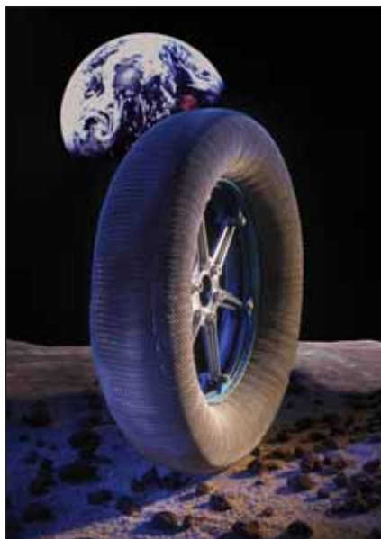
The Spring Tire , co-invented by NASA Glenn Research Center and the Goodyear Tire & Rubber Company. This airless, rubberless tire is capable of contouring to the rocky surface of the Moon, yet consumes far less energy than an Earth tire. Photo Credit — Aaron Vandersommers/Goodyear
