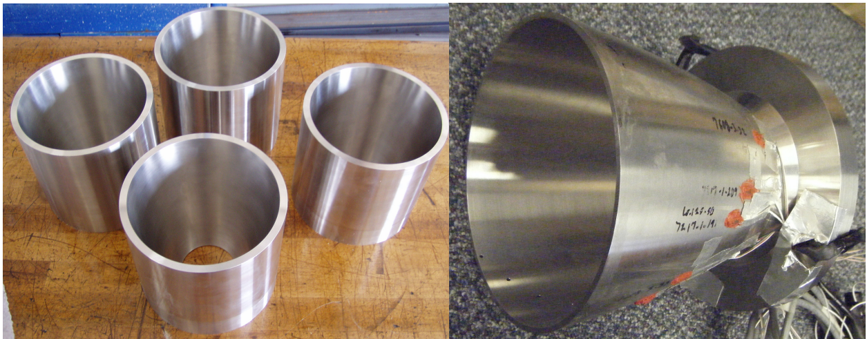
Figure 5. Hot Fire Nozzle Extensions (Left) and Instrumented Nozzle Extension (Right)
