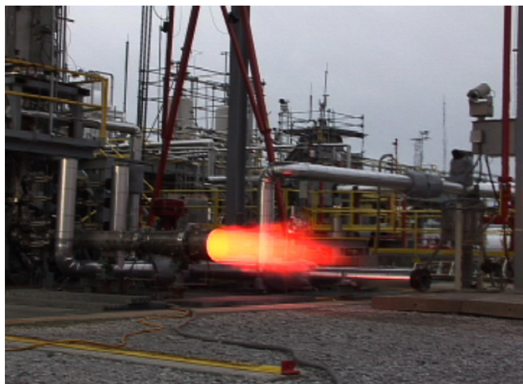
Figure 12. Afterburning During JSS Activation Testing
