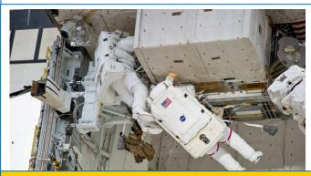
S131-E-009456 --- Mastracchio (right) & Anderson conduct 3rd & final session of EVA. Activities included fluid lines hookup of new 1,700-pound ammonia tank and prepared cables on the Zenith 1 truss for a spare Space to Ground Ku-Band antenna.
