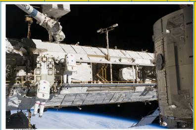
AT LEFT: S131-E-008710 --Mastracchio (left) & Anderson conduct 2nd EVA during which they unhooked and removed depleted ammonia tank and installed a 1,700pound ammonia tank on ISS Starboard 1 truss. Crew had problems with bolting down the new ATA tank on S1. They eventually got all 4 bolts secured, however, the time required to do this resulted in several tasks dropping off this EVA.
