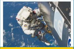
S129-E-007762 "New Dad In Space", Bresnik, installing a Grappling Adaptor to On-Orbit Railing Assembly (GATOR) on Columbus Lab. EVA 2. (21 Nov. 2009)
