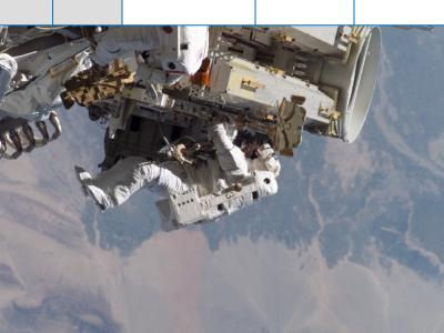
S115-E-05623 (12 Sept. 2006) --- Piper, releases the restraints on the forward Solar Array Blanket Box (SABB) during EVA with Tanner, partially visible at top edge of frame.
