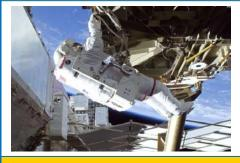
ISS021-E-030165 (19 Nov. 2009) Foreman installing a spare S-band antenna structural assembly to the Z1 segment of the station's truss. EVA 1.
