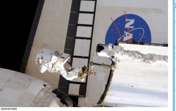
iss015e12948 -- EVA Repair: Anchored to a foot restraint on the RMS robotic arm, astronaut John "Danny" Olivas moves toward port OMS pod thermal blanket damage during EVA 3. Skin stapler and pins were used to make the repair.
