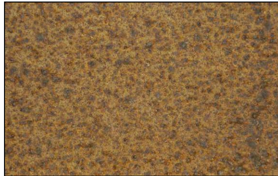
Nitric Acid, 20-25vol% + 2-3wt% \text{Na}_2\text{Cr}_2\text{O}_7 \cdot 2\text{H}_2\text{O} , RT, 75min.
