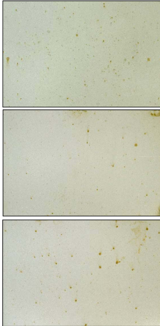
Nitric Acid, 20-25vol%, RT, 60min.
