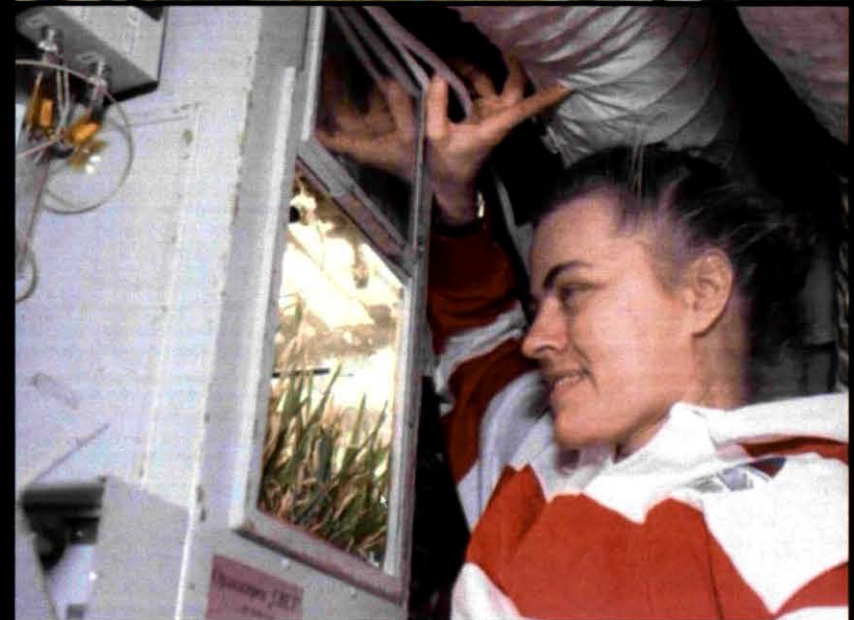
Ethylene (and VOC) scrubbing was found to be critical for successful seed production (SVET Studies).
