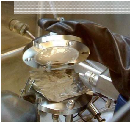
Membrane filter removal inside glove box.
