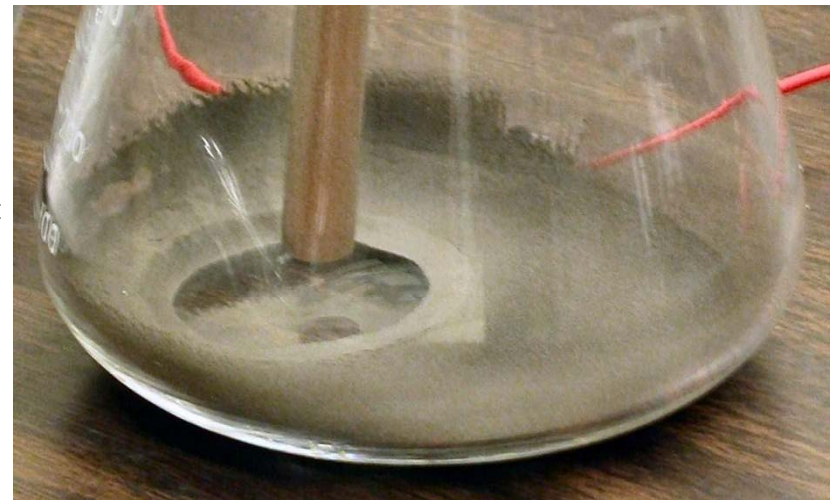
Metal tubing (copper or stainless steel) has least amount of dust adhesion of all tubing types tested.
