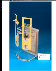
Reflectarray Antenna SCDS 615 Element Prototype + Ka-Band Space Qualifiable
