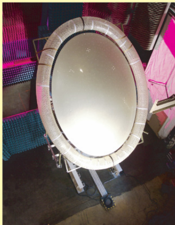
Overhead photograph of 4- by 6-m inflatable reflector in GRC near field facility
