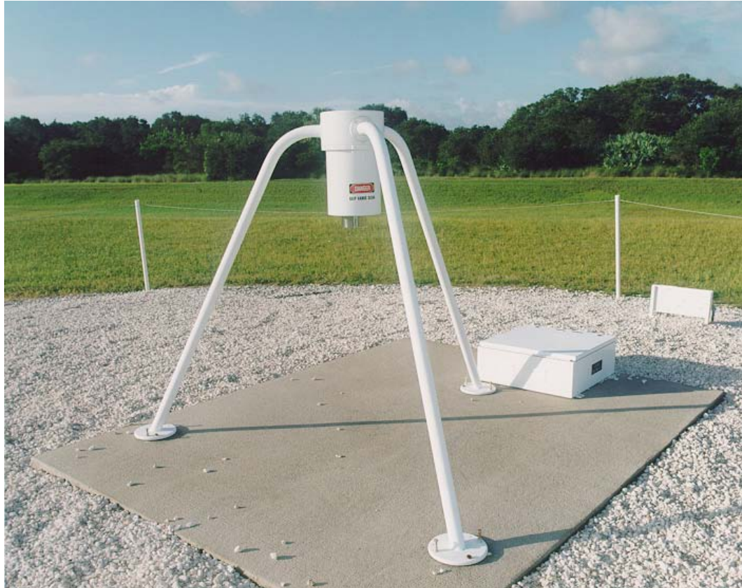
Figure A8.1.1-2 An electric field mill
