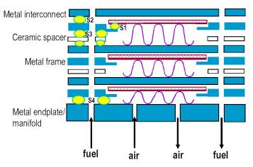
S1: PEN to Frame Ceramic to Metal Seal S2: Interconnect to Frame Metal to Metal Seal S3: Frame to Spacer Metal to Ceramic Seal S4: Frame to Endplate Metal to Metal Seal
