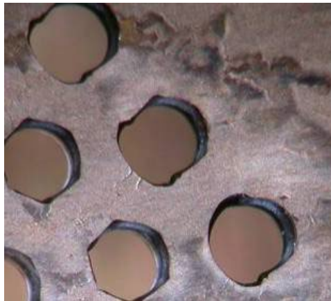
Figure 35.—Thruster PM1R accelerator grid outer apertures after the wear test.
