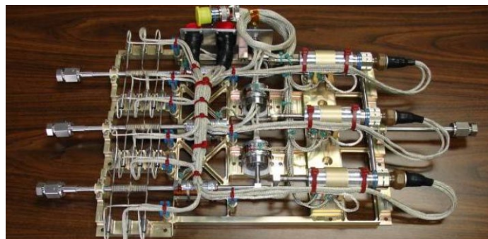
Figure 4.—Photograph of engineering model LPA.
