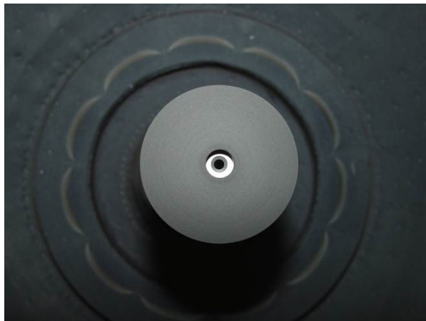
Figure 29.—Discharge cathode and keeper orifice following the wear test.
