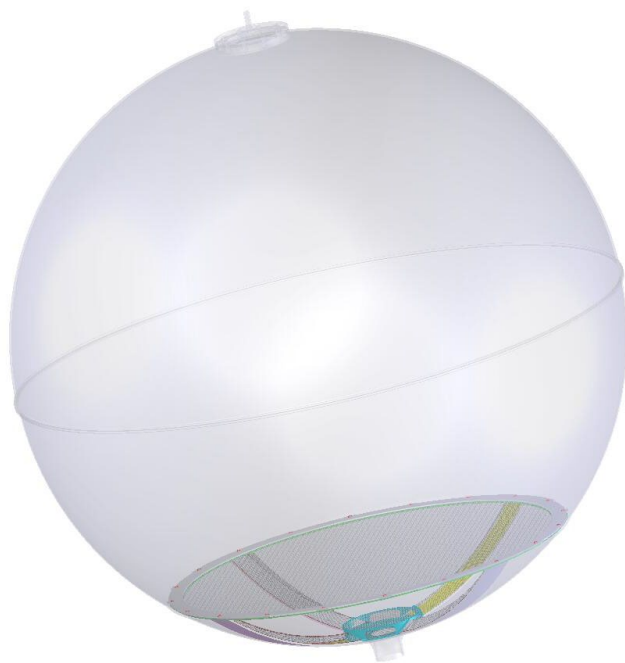
Figure 14.—Concept No. 3—Ascent stage RCS/ME partial PMD/four-channel gallery design.
