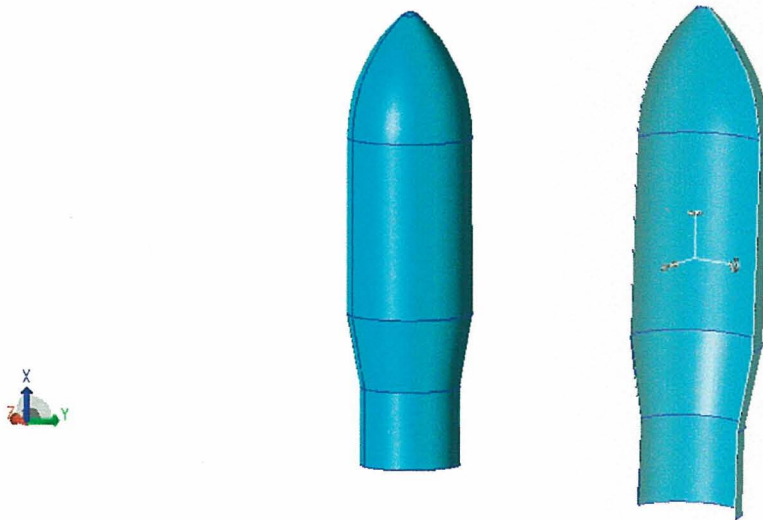
Fig. 2. ProCad WIPL-D model of fairing structure
