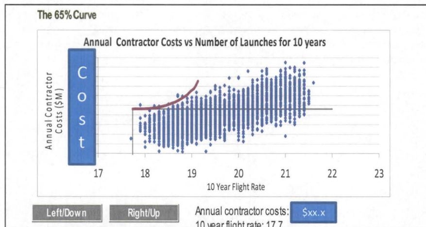
Figure 6: A sample output of the LLEGO model. Here uncertainty applies in the cost estimated by the model AND in the flight rate productivity.
